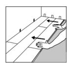
Adjust the distance to the wall to 5mm (0.2") when three rows are complete.
