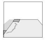
Make sure that the long sides of the planks make a straight line. Use the cut piece of the plank from the previous row to start the next one. However, it must be at least 30cm (12") long. If the piece is too short, start with a new board and cut it in half. Always ensure that the end joints are staggered at least 30cm (12").
