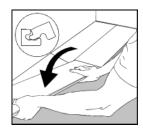
Place the short end of the plank at an angle against the previous installed plank and fold down.
