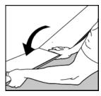
Hold the next plank against the first at an angle to the first one and lay it flat on the floor.
