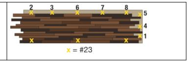
**Step 7:** Repeat the gluing procedure (step # 4) Insert the second panel in the previous one using the horizontal adjustment section. Repeat step #6.
