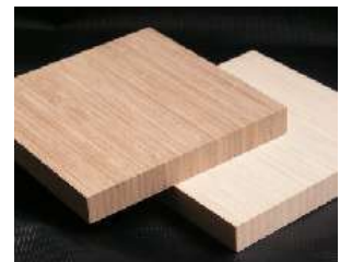
Laminated bamboo into 'stock' material
